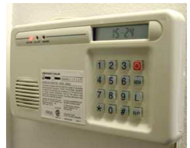
The control unit (above) will call the concierge if a sensor sends a signal. Up to five other phones can be programmed. At left is the sensor. When water is detected it sends a signal to the controller. The alarm then goes out.
