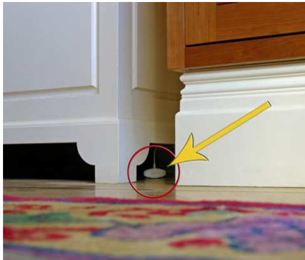
This is the cats-eye view of the sensor. The sensors are wireless and battery operated.
