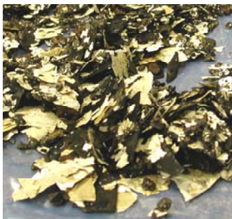
These paint chips came from the improperly painted cooling tower. It has taken three years, but they are now almost completely flushed from the system.
